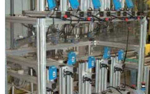
Pivot wear test rig for testing the pivoting wear rate for medium loads.
