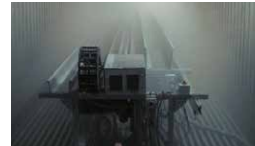
Cold test at -40 °C for chainflex ® cables and e-chains ®
