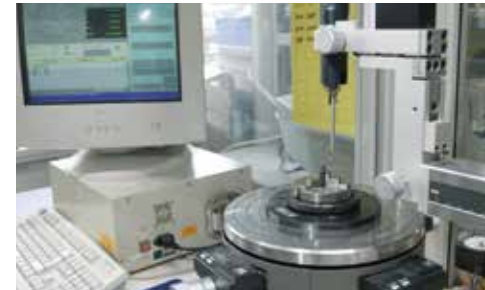
Measuring the inner diameter of a press-fitted bearing.
