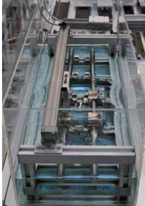
Service life and wear test of a drylin ® linear guide in the "under-water basin".
