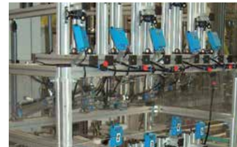
Pivoted wear test to determine the wear behaviour of iglidur®
