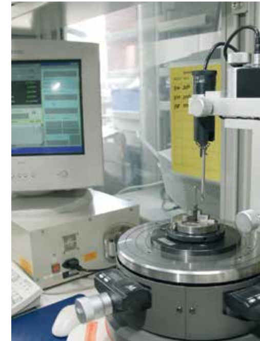
After press fitting, measurement of the inner diameter
