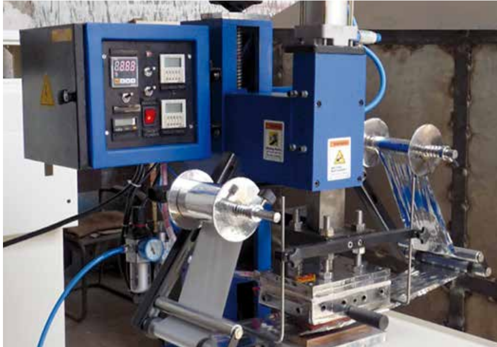
Hot foil stamping machine with drylin® drive technology
