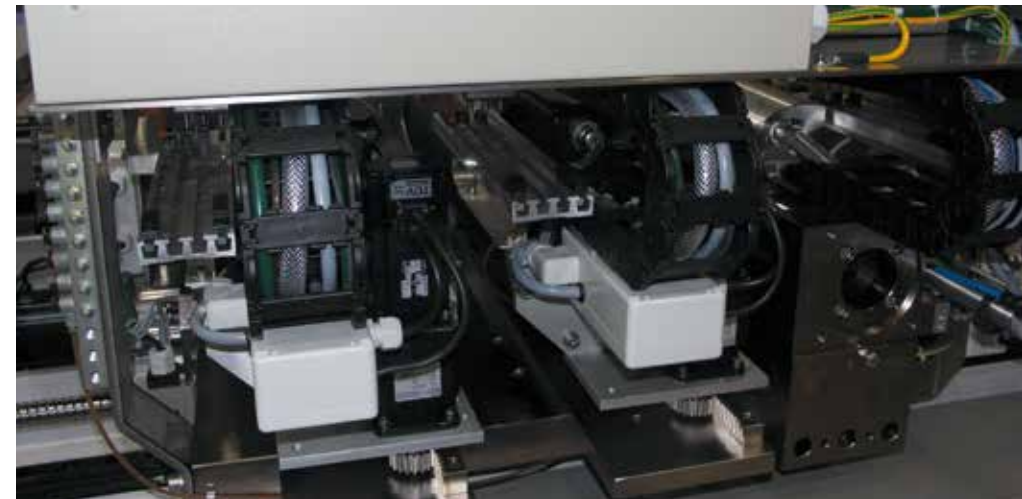
e-chain® and chainflex® cables in special machine construction for gravure printing
