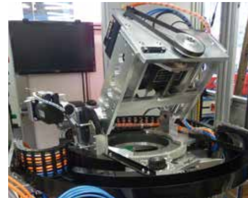
Engraving machine with circular-mounted igus® e-chains®
