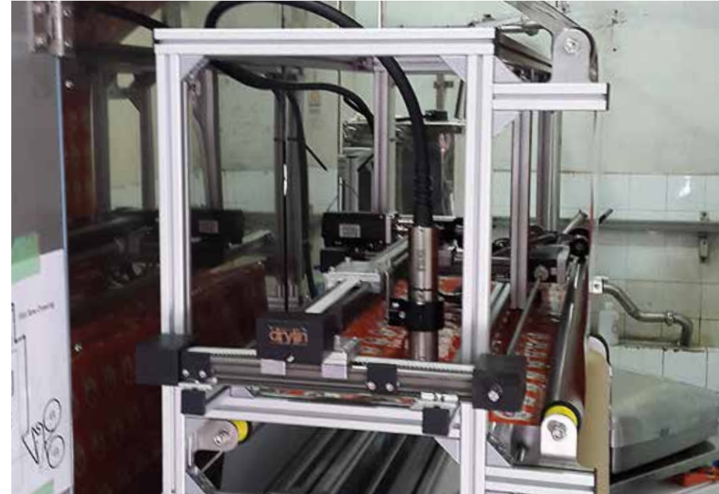
drylin® toothed belt axes as flat gantry in a printing system
