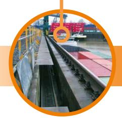
The first igus® rol e-chain® in Europe with a travel of 130 metres as the main way of supplying power to a crane system.
