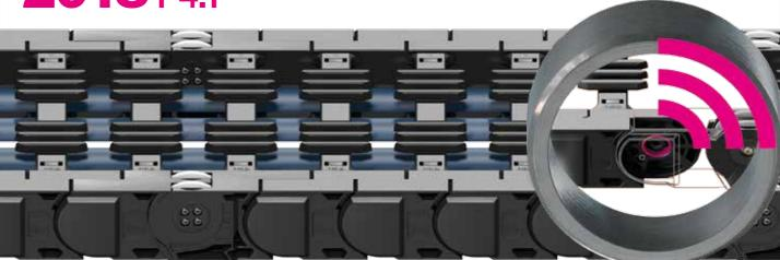
In the latest development stage of the igus® rol e-chains®, the use of maintenance-free, tribo-polymer plain bearings in the connection of the e-chain® links also considerably lengthens the service life. As an option, they can also be fitted with wear sensors, to reliably predict the expected service life of the system. Compared to the first rol e-chain®, the expected service life has been more than trebled.
