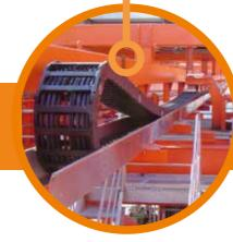
Heavy-duty rol e-chain® in a STS crane. The "HD version" of the rol e-chain® becomes the standard for STS crane applications and ship loaders/unloaders with long travels and high speeds, worldwide.
