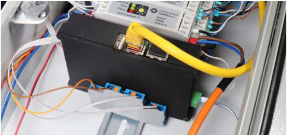
Figure 4.6: Embedded Computer with Ethernet cable connected to the ETH0 socket.
