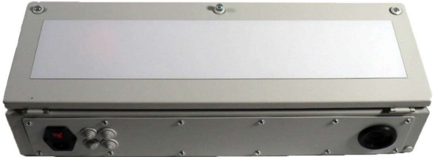
Figure 4.4: Control Cabinet, closed. On the lower left the mains IEC connector / switch / fuse and the cable fittings can be seen.
